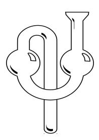
A glass or plastic fermentation lock -a curlicue stopper-fits into the neck of the bottle and prevents air from contaminating the cider while allowing fermentation gasses to escape.
